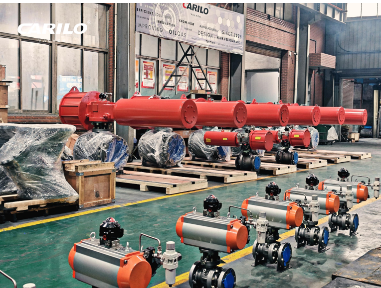
Casting trunnion mounted ball valve, 3" 300LB, soft seated, CS/SS, Forged trunnion mounted ball valve, 16" 300LB, soft seated, CS/SS, Pneumatic, offshore, Argentina
